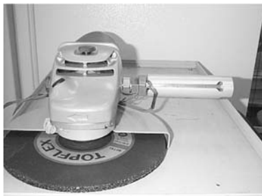
Fig. 11 9" angle grinder equipped with a force measurement handle
